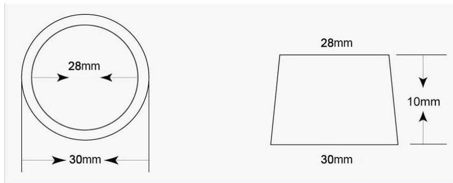
Figure 2: M10 Stud - Top and side view
