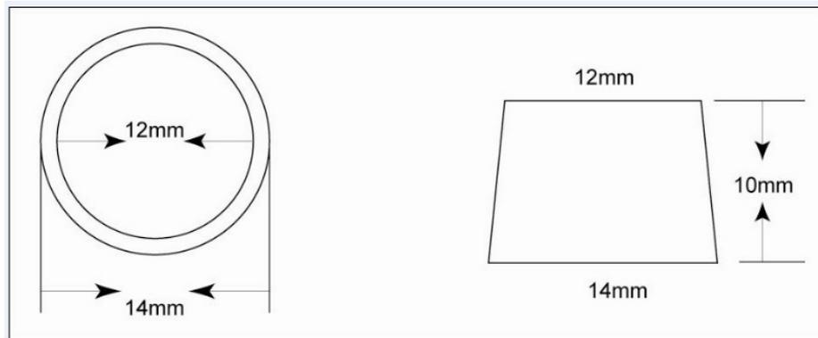
Figure 1: M5 Stud - Top and side view
